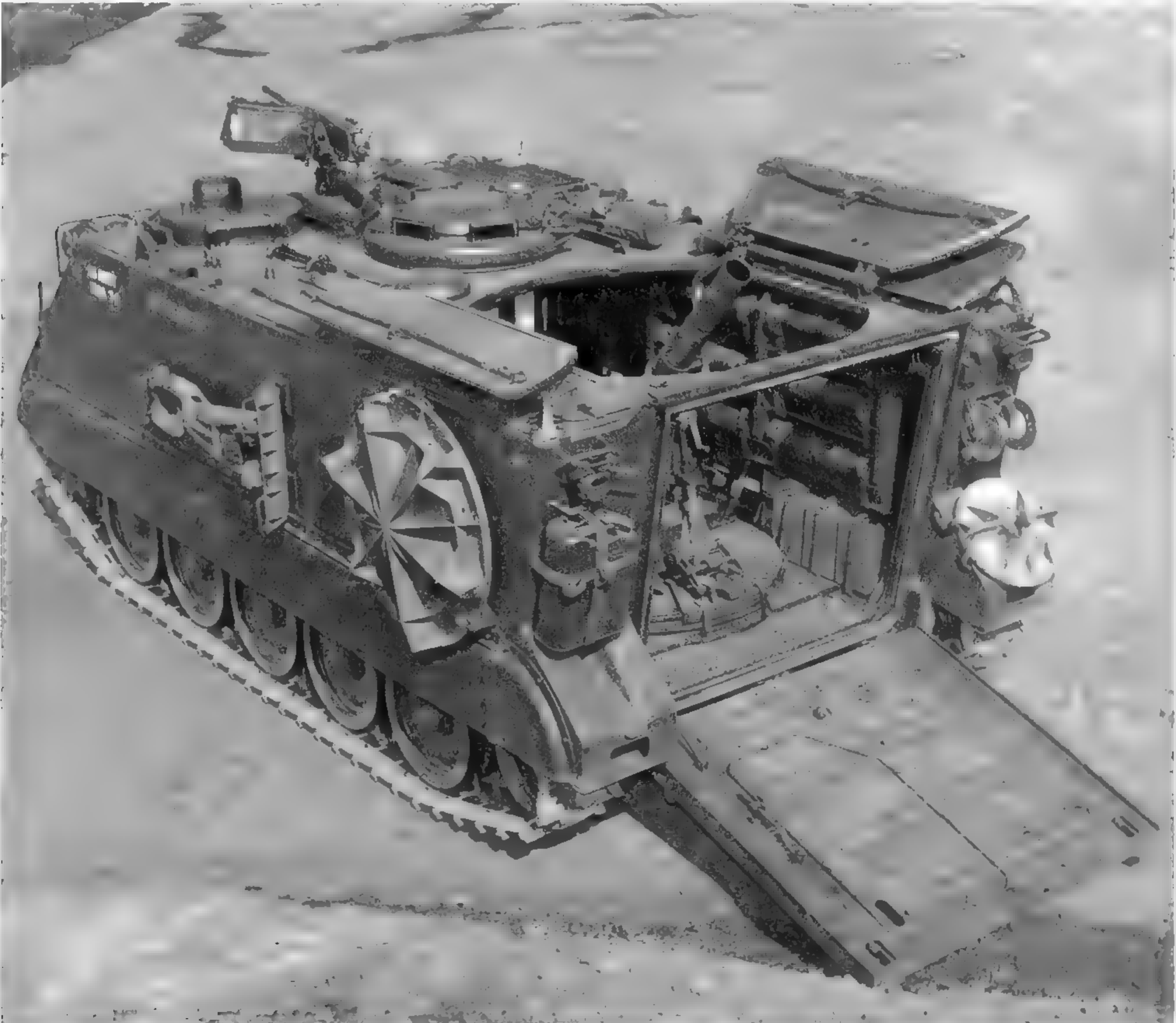
The 107mm mortar of the M106-series mortar carriers could be dismantled from the vehicle and, using the base plate assembly secured to the side of the hull, be fired from a fixed position. This allowed the vehicle to be used for other purposes. This M106A2 is in firing position with the roof hatches open. Mortar rounds can be seen stowed in the ammunition racks inside the vehicle. (U.S. Army photo)
